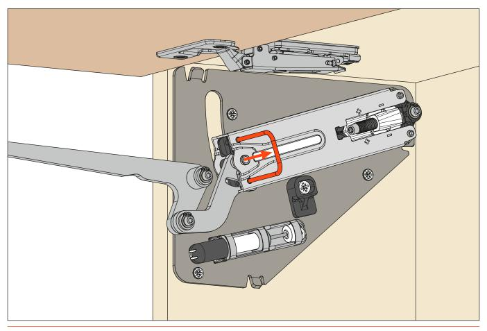
Adjustment of the system strength. Use a Torx bit T20.
