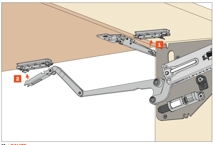
Withdraw the safety clip. Lower the door slightly until the safety clip can be easily withdrawn.
