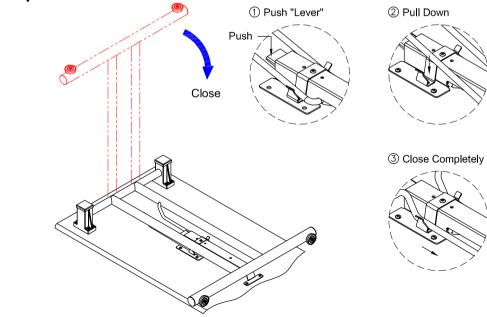
★ Caution: Make sure to push "Mechanism Lever" before pulling down the frame to closed flat position.
